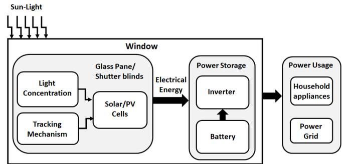
Fig. 4: Block diagram of an Advanced Solar Window
