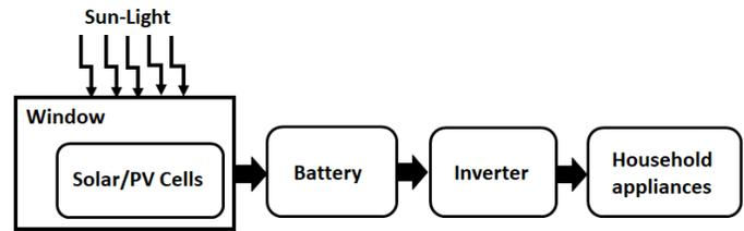
Fig. 3: Block diagram of a Traditional Solar Window
