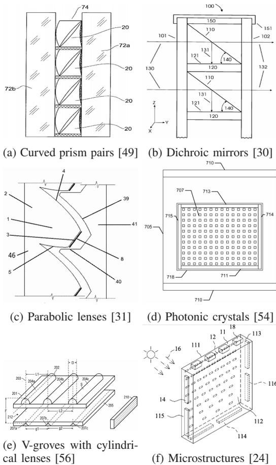
Fig. 5: Different optical elements used for Light concentration
