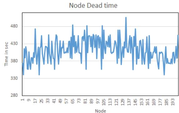
Fig. 4: Time taken by nodes to die in Leach
