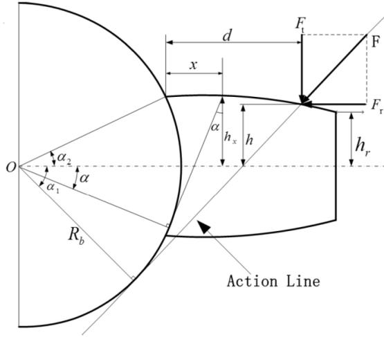
**Figure 1** Schematic diagram of spur gear tooth model [3]
