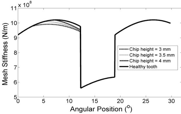
Figure 6. Effect of chip height on TVMS of gear pair
