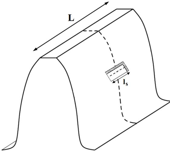
Figure 4. Schematic diagram of spalled tooth
