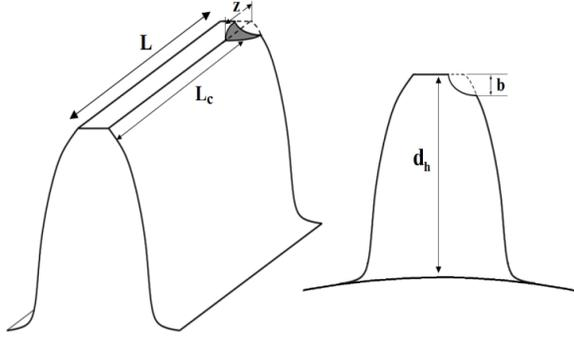
Figure 3. Schematic diagram of chipped tooth
