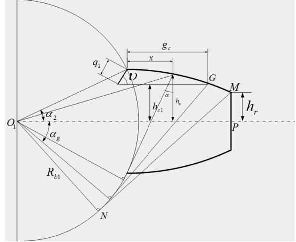
**Figure 2** Schematic diagram of cracked tooth [3]
