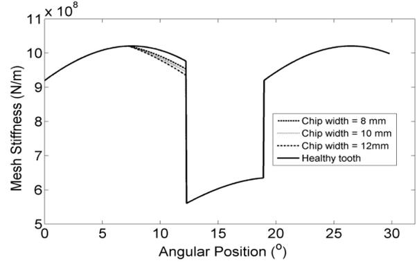
Figure 7. Effect of chip width on TVMS of gear pair
