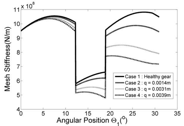
Figure 5. Effect of crack length on TVMS of gear pair
