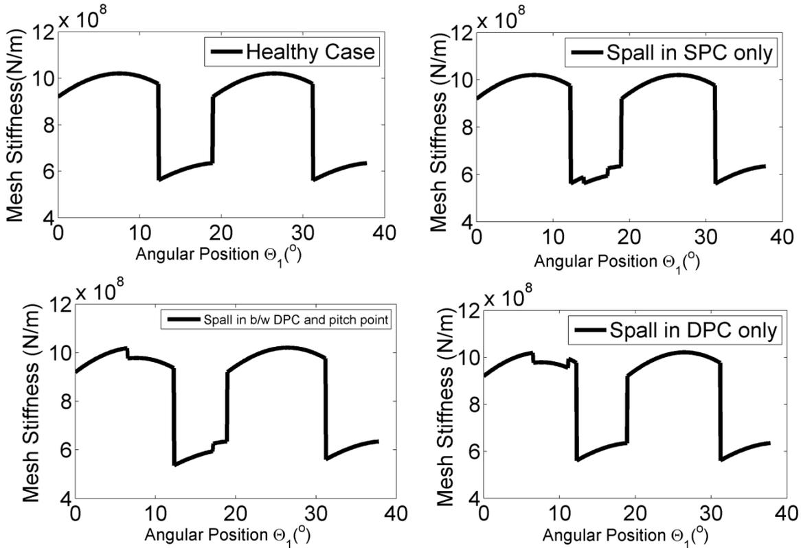
Figure 8. Effect of spall position on TVMS of gear pair
