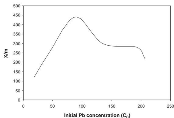
Fig. 5. Variation of lead loading with initial lead concentration.
