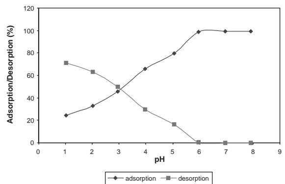
Fig. 6. Adsorption and desorption of lead by sea nodule at varying pH.
