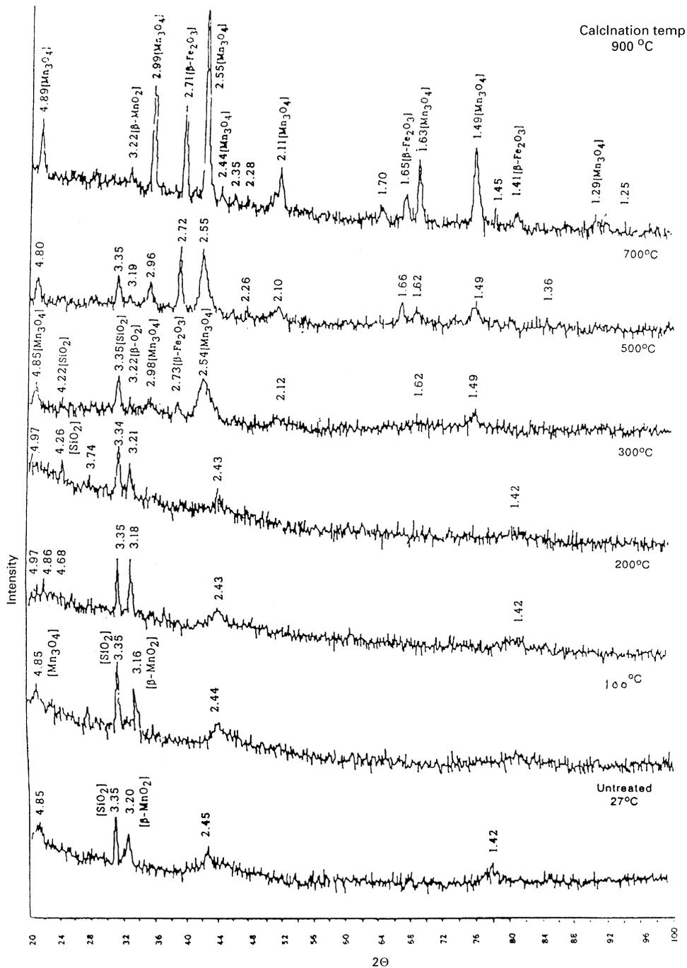
Fig. 7. X-ray diffractograms of various calcined products of sea nodule.
