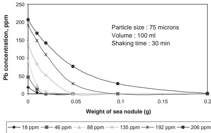
Fig. 3. Pb adsorption profile of sea nodule.
