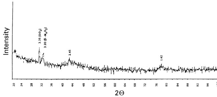
Fig. 2. X-ray diffractogram of sea nodule.
