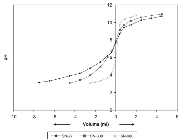
Fig. 8.  $pH_{zpc}$  curves of various calcined products of sea nodule.
