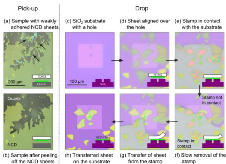
the diamond film from this substrate. During the growth, these materials expand at different rates creating stresses that split one layer from the other.
